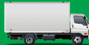
6-WHEEL TRUCK • 5 TON • 24 M 3 LxWxH: 500x220x220 CM
